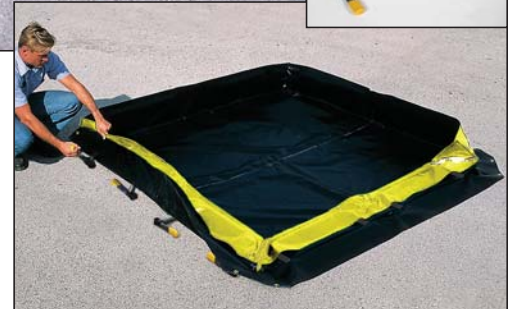
Simply swivel the “feet” of the PVC supports to lower the sidewall. Vehicles and equipment can then roll over the top of the collapsed wall for convenient entry and exit.
